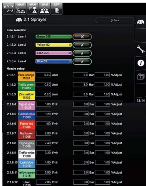
This setup shows that utilising all four nozzles can give a theoretical speed range of 3.0 to 27.1km/hr at 100 litres/ha in a 1.8 to 4 bar pressure range.
