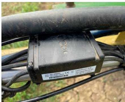
The system seems complex, but INC 2.0 controllers are simple plug-and-play units with flashing LEDs to highlight any errors in the setup.
