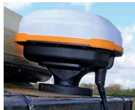
GPS and algorithms are used to calculate how tight the vehicle is turning and how fast each section of the boom is travelling in relation to that.
